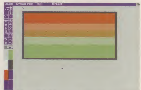
This image shows how you can alternate colours in a crosshatch pattern to give the impression of there being more colours on screen than there actually are.
